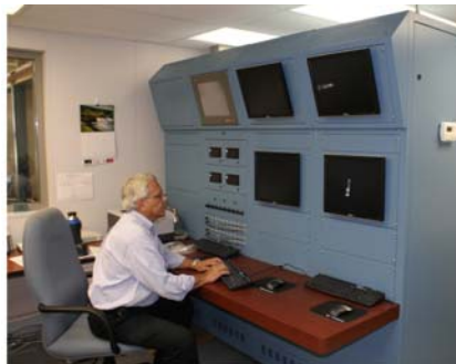
The data acquisition system collects the mechanical and aerodynamic information for analysis and storage.
